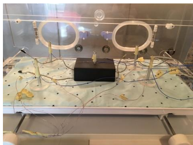
Figure 6 Incubator temperature measurement using thermocouple K-type and T-type.
