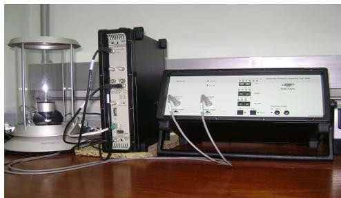
Gambar 1 Sistem Kalibrasi *Reciprocity* Tipe 9699 Berbasis Pulse (Generasi Keenam)
